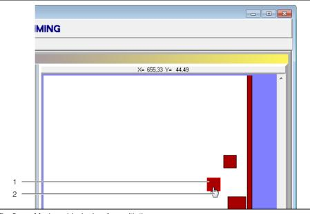
Fig. 8: Moving a blocked surface with the mouse
