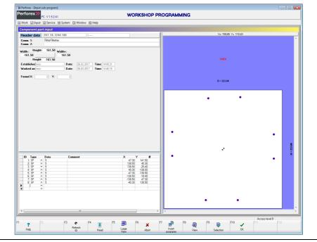
Fig. 26: Component part with predrilled holes
