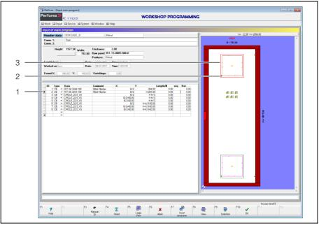
Fig. 9: Selected component part in the line data and the graphical representation
